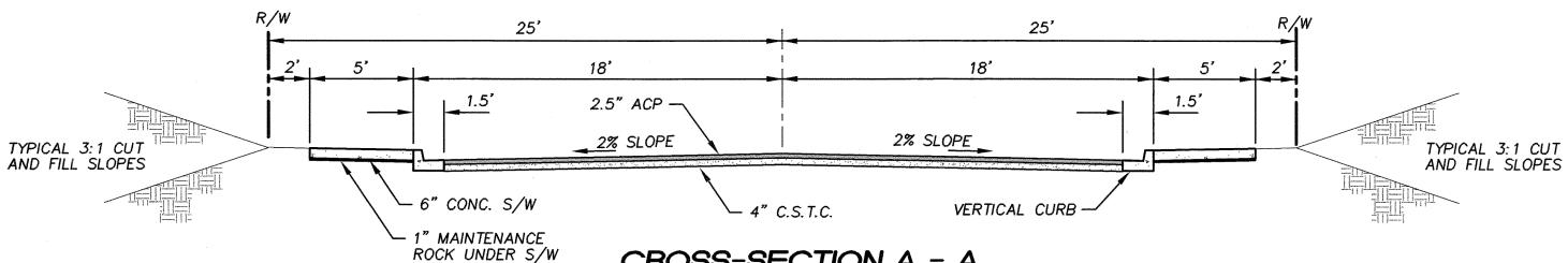
CROSS-SECTION A - A SCALE 1" = 5"
