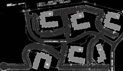
This site and the local weather created difficult issues to deal with in the design. The site is a peat bog, and contained possible "Ice Lenses". Sonic testing was used to locate these lenses and remove them. The buildings were supported by pilings and designed to withstand high earthquake loads. The severe ranges of temperatures between the frozen winters and hot summers also presented design challenges. The project is 25 years old this year and has withstood these challenges well.
