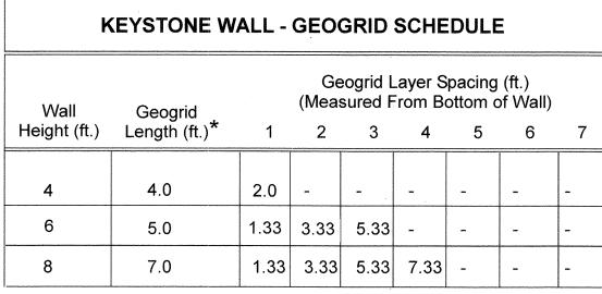
\* NOTE: Geogrid length shall be measured from back of wall.
