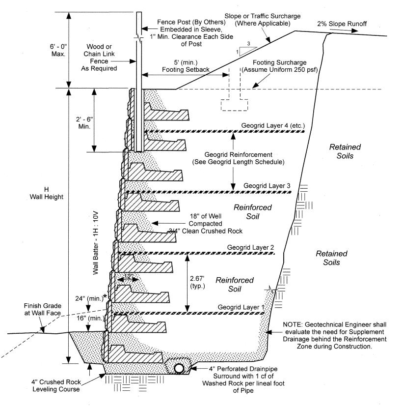
\*NOTE: Wall Toe cover shall be 24" (min.) for Sloping Condition in Front of Wall and at Detention Pond
