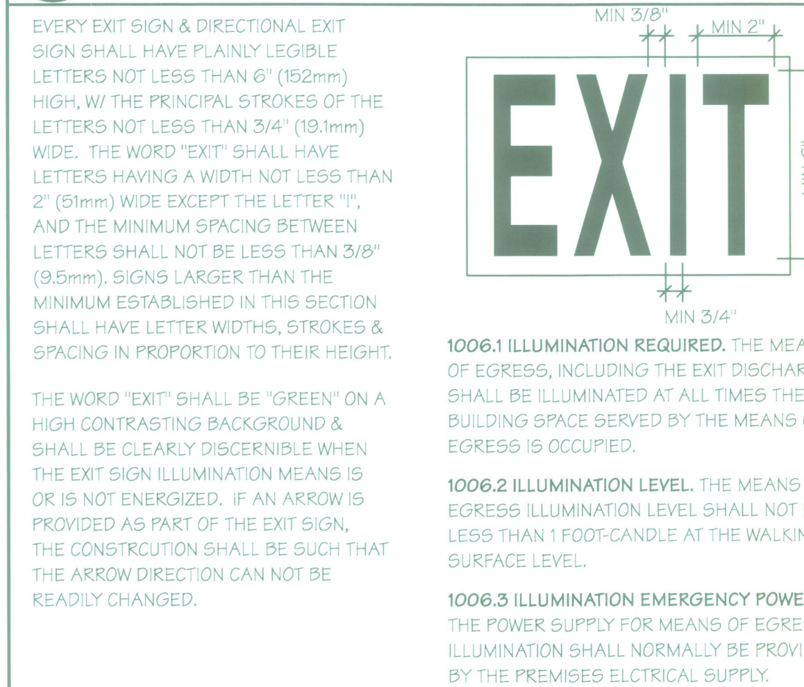
10 EXIT ILLUMINATION SIGN SCALE: 3" = 1'-0"
